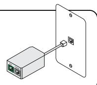
Plug either end of the green phone cable into the green "DSL" port of the splitter.
